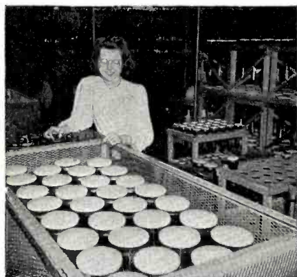
Final inspection of television tubes in the Sylvania plant.
